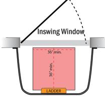
Minimum size window well for both a slider and inswing style window are  $42^{\circ}$  x  $36^{\circ}$  with a Life-Step<sup>TM</sup> ladder.
