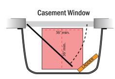
Recommended minimum size areawell for a casement style window is 50" x 36" with a Corner-Step  $^{\text{TM}}$  ladder.
